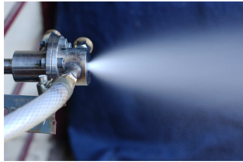
Figure 5. Coaxial injector using water/air as simulant
